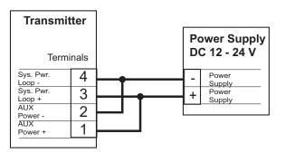
Connection to a PLC/Recorder, separate supply
